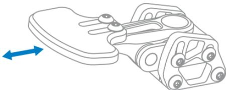
Reach can be adjusted by slightly loosening the two screws highlighted in the right picture and the two on the opposite side of the shifter as pointed by the small arrows, then rotating the lever body upwards/downwards. You may need to apply a bit of force.
